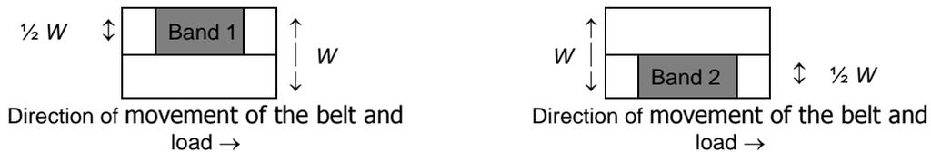
In figure 5.2-1,  $W$  represents the width of the load transport system if there are no guides or width between guides where they exist.
