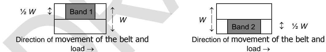
Figure 5.2-1: Positions of load for test of eccentricity.
